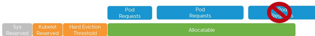
Scheduling of Pods with Requests and "Node Allocatable"
